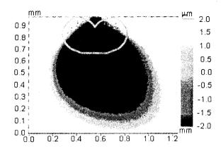
Figure 6: Theoretical plastic zone at K=30 MPa•m<sup>1/2</sup> compared to surface deformation at same K level
