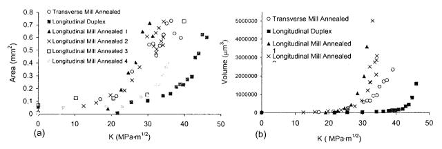
Figure 3: Deformation and stress factor relationship for Ti-6Al-4V for (a) area and (b) volume
