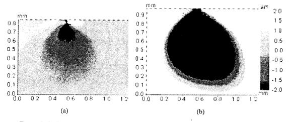
Figure 5: Deformation zones under loads of (a) 2500 N and (b) 3500 N (directly before failure)
