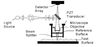
Figure 2: Schematic of White Light Interference Profilometer
